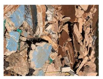
Construction and Demolition Waste - sorted without reinforcement
